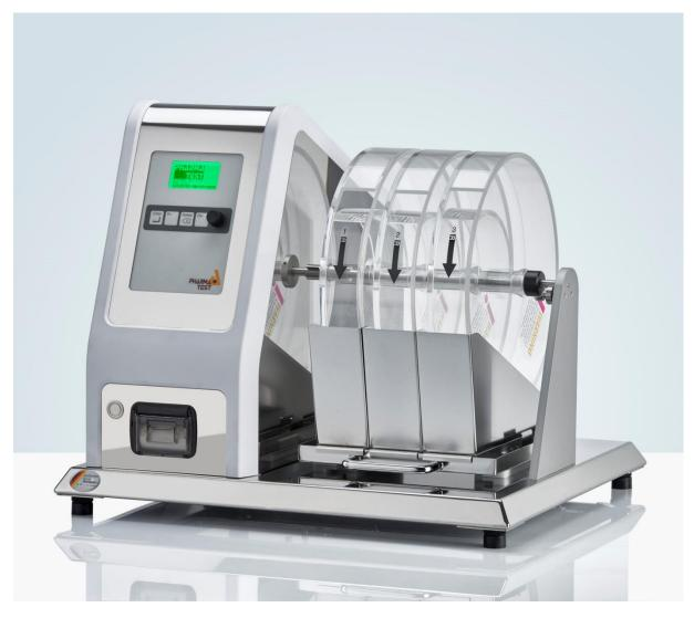
One of the testing criteria for mechanical strength of tablets and cores according to the USP <1216>, EP <2.9.7>, JP <14> and other pharmacopoeia is friability and abrasion testing. During the process of coating, transportation and packing the tablet will lose some amount of weight. To measure this weight loss, the samples are counted and weighed. Then the friability test is performed following the individual monographs of the relevant Pharmacopoeia. The tablets are tumbled at each turn of the
